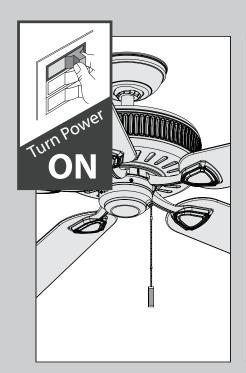
The pull chain controls the fan: high, medium, low, extra low, and off.
