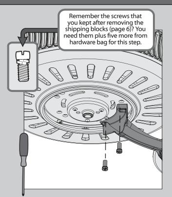
Lightly attach the blade irons to the motor with screws found in the ∑ hardware bag, then securely tighten after both screws are attached.
