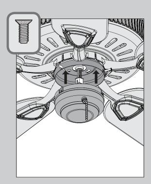
Lift the lower switch housing up until the holes line up with the screw holes in the upper switch housing. Install the three (3) switch housing screws, found in the ≡ hardware bag.
