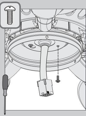
Insert the third screw, found in the ≡ hardware bag, into place and then tighten all three (3) screws.
