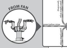
Using an orange wire connector from the hardware bag, connect the 3 grounding wires (green, green/yellow stripe, or bare copper) coming from the ceiling, downrod, and hanging bracket.
