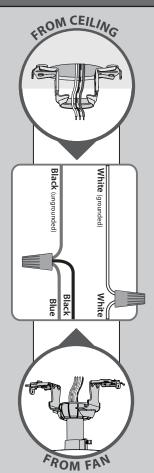
Using orange wire connectors from the hardware bag, connect the black wire (ungrounded) from the ceiling to the black and the blue wires from the fan. Connect the white wire (grounded) from the ceiling to the white wire from the fan.
