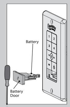
To change the battery, push on the battery door to eject it. Remove the battery using a small Phillip's head screwdriver. Replace with same type battery, making sure the (+) side is facing down. Replace battery holder and battery door.
