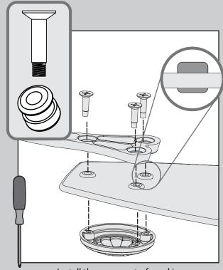
Install the grommets, found in the hardware bag, in the blades by hand. The thicker ends of the grommets should face upward toward the blade iron. Place each blade between a blade iron and medallion. Install three blade screws, found in the hardware bag, to attach the medallion to the blade iron. Repeat for all blades.
