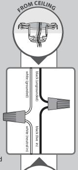
Turn the splices upward and push them carefully back through the hanger bracket into the outlet box. Spread the wires apart, with the grounded wires on one side of the outlet box and the ungrounded wires on the other side of the outlet box.
