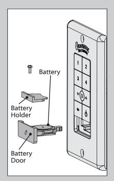
Before operating the wall control, press on the battery door to eject it. Unscrew the battery holder. Insert the battery, found in the control hardware bag, with the positive (+) side facing downward. Reinstall the battery holder and reinsert the battery door into the wall control.
