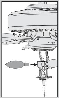
Install a light bulb in each socket.
