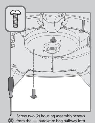
the motor housing. It does not matter
