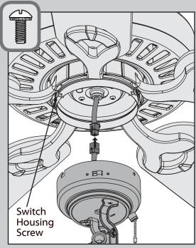
screws found in the ≡ bag. Connect the plugs from the upper and lower switch housings. Make sure to line up the colored markings on the connectors.
