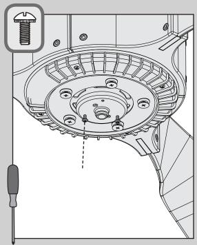
Screw two housing assembly screws from the hardware bag halfway into the motor housing. It does not matter which two screw holes you choose.
