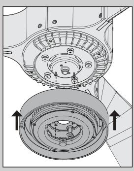
Wrap keyhole slots around the screws and twist counterclockwise.
