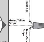
Using an orange wire connector from the \* hardware bag, connect the 3 grounding wires (green, green/ yellow stripe, or bare copper) coming from the ceiling, downrod, and hanging bracket.
