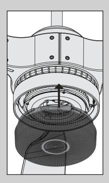
Lift the globe and align the notches in the globe with the tabs in the light kit. Attach the globe by lifting and twisting clockwise until it rests firmly in place.
