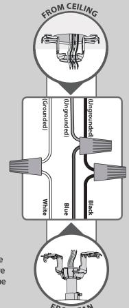
Turn the splices upward and push them carefully back through the hanger bracket into the outlet box. Spread the wires apart, with the grounded wires on one side of the outlet box and the ungrounded wires on the other side of the outlet box.
