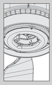
Connect the white wire from the fan to the white wire from the light kit. Then, connect the blue wire from the fan to the black wire from the light kit.
