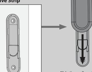
Slide the cradle onto the mounted bracket.
