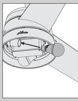
Install a bulb into each of the sockets. When necessary, replace with bulbs of the same wattage.
