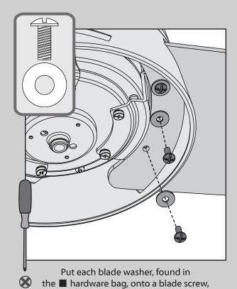
found in the  $\blacktriangle$  hardware bag. Then secure each blade to a blade iron using the blade screws and washers.
