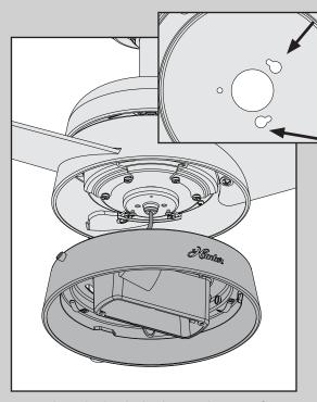
Align the keyhole slots in the top of the light kit assembly with the partially installed assembly screws. Wrap the keyhole slots around the screws and twist counterclockwise.
