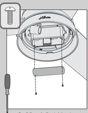
Carefully push all switch housing components into the switch housing, then install the switch housing plate using two light kit assembly screws, found in the ≡ hardware bag.
