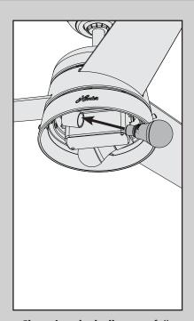
Changing the bulbs - carefully remove the globe. Unscrew the bulbs and replace them with bulbs of the same wattage.
