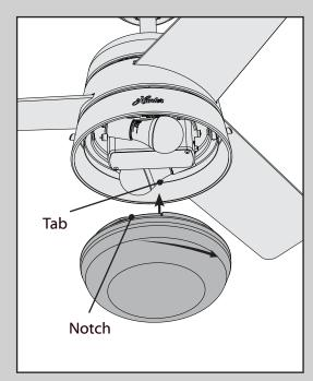
Align the notches in the outer rim of the globe with the tabs on the light kit assembly Carefully lift the globe up inside the light fixture as far as it will go. Rotate the globe in a clockwise direction until it is held tightly in place by the three tabs.
