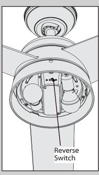
Changing the direction of air flow - carefully remove the globe and move the reverse switch to the opposite position.
