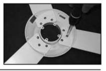
(10) Reinstall rotor using the four rotor screws from step (7). Be sure screw tabs on rotor are properly aligned with correct holes on motor.
