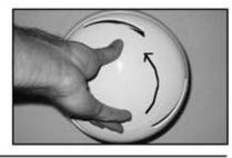
(7) Disassemble rotor from fan motor by removing the four rotor screws as shown. Keep rotor screws for reinstallation in step (10).
