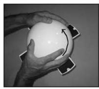
(7) Carefully insert blades into rotor slots, and using screws from hardware package, secure blades to rotor. The counter sink screws ("blade center screws") are for the single blade hole outside the rotor and the pan head screws ("blade holder screws") are for the two holes inside the rotor area.
