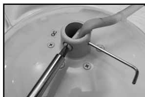
Remove stopper screw & loosen hex screw
