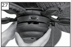
Attach switch housing cover onto switch housing by aligning the long slot on switch housing cover with the reverse switch preassembled on switch housing as shown.
