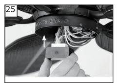
Attach capacitor onto switch housing by preadhered doublesided foam tap as shown.
