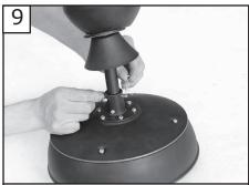
Insert downrod into the yoke on top of fan body. Align the hole in the downrod with the hole in the yoke. Insert cross pin through yoke and downrod until point appears on the other side.
