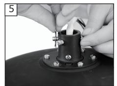
Remove keeper pin and cross pin from yoke, and save for later use.
