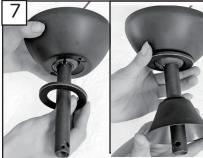
Place canopy bottom cap over downrod and then place yoke cover over downrod as shown.
