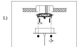
Step.1: Remove mounting bracket (A) from fixture and install to electrical box.
