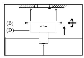
Step3: Install fixture to bracket and Screws at the ends of the canopy to secure.
