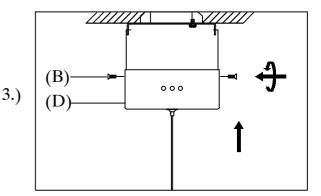
Step3: Install fixture to bracket and Screws at the ends of the canopy to secure.
