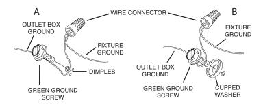
6) Make wire connections. Reference chart below for correct connections and wire accordingly.
