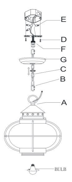
Attach appropriate amount of chain to loop to achieve desired mounting height.
