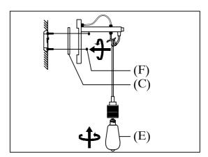
Step3: Install fixture to bracket and tighten screws at the ends of the canopy to secure. Install bulb into socket.
