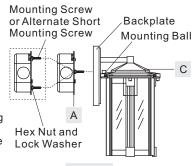
Assembly (A) by unscrewing the preassembled hex nut and lock washer and then screwing the mounting screws or alternate short mounting screws in or out of the crossbar until the correct length is achieved. Once the backplate on Fixture Body (C) is secure, remove the mounting ball and Fixture Body (C) and proceed to Step 4.
