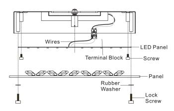
C. Connect the Live Wire from LED Panel to the corresponding port of the Live Wire from Driver. Connect the Natural Wire from LED Panel to the corresponding port of the Natural Wire from Driver.
