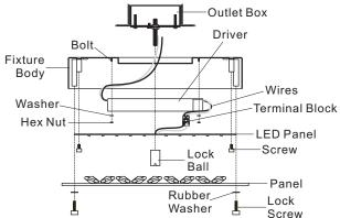
C. Connect the Live Wire from Driver to Port "L" on the Terminal Block, which is the corresponding port of the Live Wire from LED Panel. Connect the Natural Wire from Driver to Port "N" on the Terminal Block, which is the corresponding port of the Natural Wire from LED Panel.
