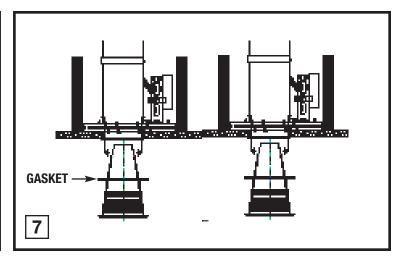
**FOR 1154 TRIMS:** Before installing trim, remove socket plate from housing by loosening wing nut. Unfasten socket from socket plate by squeezing springs and snap into hole provided in top of trim (see Diagram 5). If using 1155ATR (See Diagram 7). Discard socket plate / bracket.
