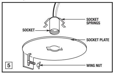
**FOR ATR TRIMS:** Before installing trim, remove socket plate from housing by loosening wing nut. Unfasten socket from socket plate by squeezing springs and snap into hole provided in top of the trim or reflector. Install trim by pressing reflector around lip of trim and turn clockwise to lock into position.
